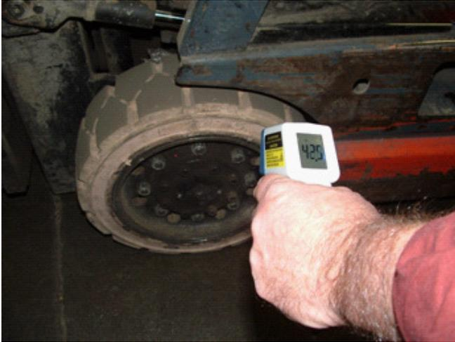
To measure heat in the actual tire, aim infrared digital thermometer at several spots on the tread and sidewall of the tire. Unless there is a wide variance of temperature, record the highest temperature reading.
