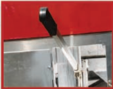
HYDRAULIC HAND PUMP is located on the side of ramp. It raises the top of ramp from 38" to 61"
