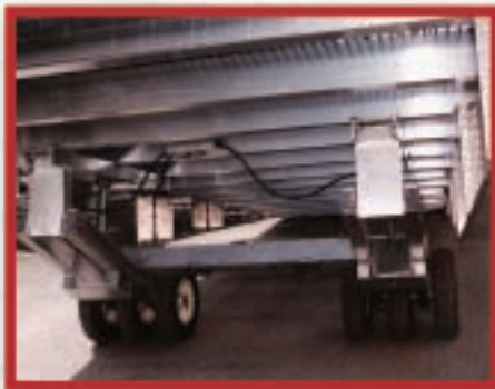
UNDERSTRUCTURE consists of a rigid double channel box section aluminum frame carrying six wheels and is hydraulically lifted.
