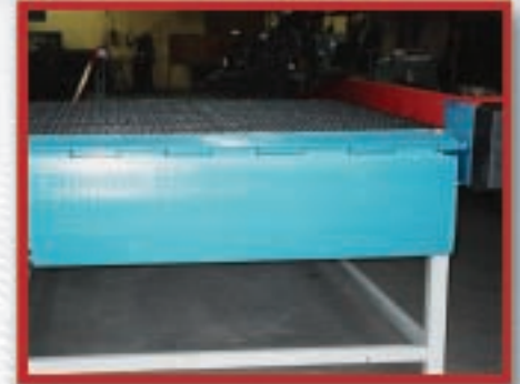
PICTURED ABOVE is the edge of dock in the down position and the six foot the level off section enabling a forklift to enter a truck with the forks parallel to the floor.
